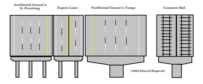
The 2025 Howard Frankland Bridge span is designed for commuter rail addition by utilizing two lanes of the express lanes and constructing a set of express lanes onto the existing 1991 Howard Frankland Bridge span. An alternative would be to construct a fourth Howard Frankland Bridge span within the footprint of the original 1960 Howard Frankland Bridge. The diagram shown above reflects construction of that fourth Howard Frankland span instead of adding on to the 1991 span.
